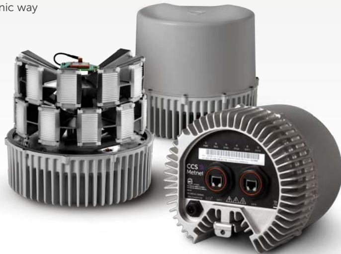
The Metnet system operates in a single frequency channel with no radio frequency planning required. Frequency reuse in the entire network is 1. Each node has a wide 270-degree field of view, so only one unit is required per site, rather than multiple radios. There's no need for any manual alignment and each node supports multiple connections for higher resilience.
